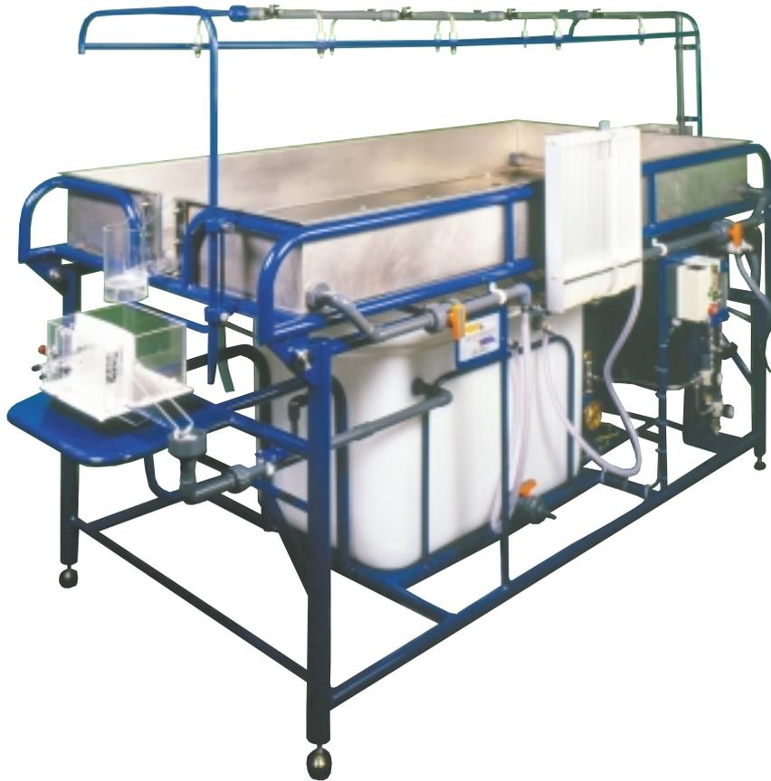
*This apparatus demonstrates some of the major physical processes found in hydrology and fluvial geomorphology, including: rainfall hydrographs for catchment areas of varying permeability; the abstraction of ground water by wells, both with and without surface recharge from rainfall; the formation of river features and effects of sediment transport.*
