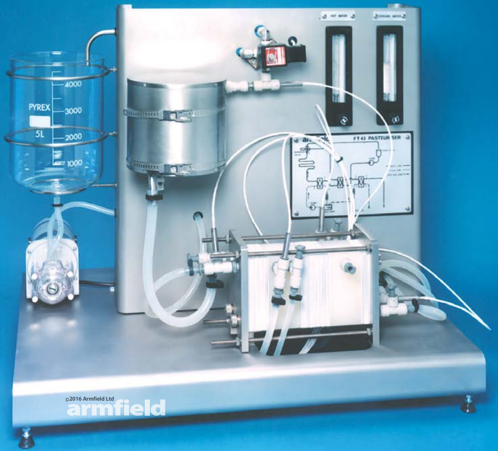
FT43 Laboratory Pasteuriser showing 45-second holding tube installed
