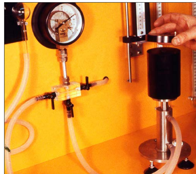
Calibration of a Bourdon gauge using a deadweight calibrator
