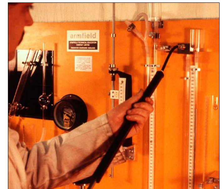
Pressurising a manometer
