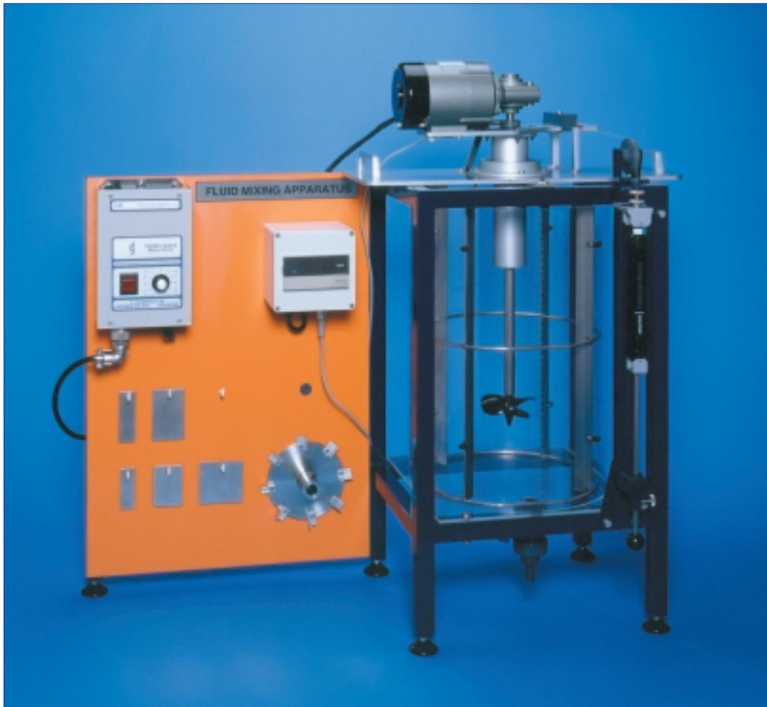
*The Armfield Fluid Mixing Apparatus has been developed to demonstrate the factors affecting mixing using visualisation and measurement techniques as appropriate. It is suitable as an instructional aid or as a design tool for large scale mixers.*
