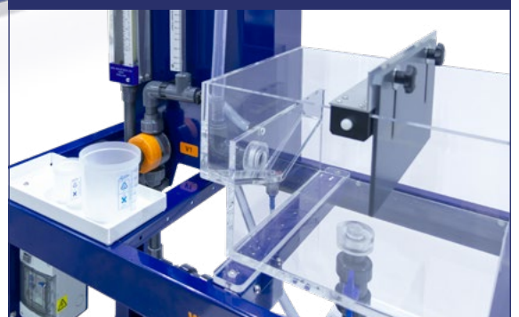
Water and slurry flow meters
