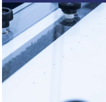
Flow straightener and dye injection system
